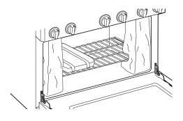
**ACAUTION** Doors and passageways leading to the installation location require at least 32" opening. If the opening is less than 32", the oven door(s) and control knobs must be removed.
