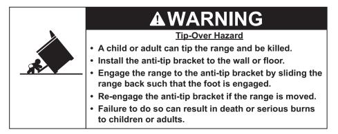
To reduce the risk of tipping the range, the range must be secured by a properly installed anti-tip bracket. See installation instructions shipped with the bracket for complete details before attempting to install.
