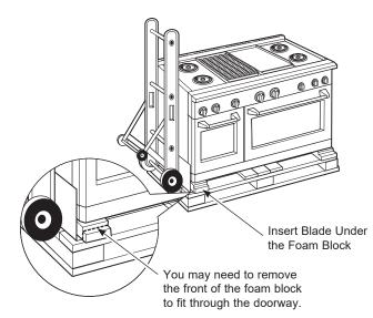
**IMPORTANT:** Do not remove the base foam block while the hand-truck is in use. Place the hand-truck blade underneath the base foam block and transport the range to the final location. 4. Attach the hand-truck straps around the unit.
