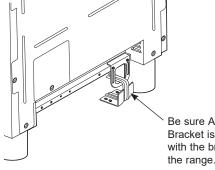
Be sure Anti-Tip Bracket is engaged with the brace on
